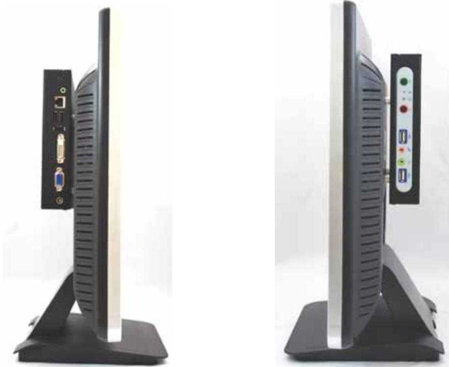
The areas of design and handling are well thought through by the manufacturer. In our test, we tried to run the mainboard completely cooled passively and the combination of mainboard and case passed this test with honors. We had this combination run for 48 hours with a full work load and we couldn't recognize any decrease in performance.
